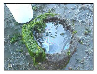
Figure 1. Creosote compounds leaching from an old piling in South Fidalgo Bay.
