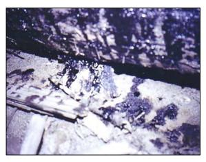
Figure 2. Creosote compounds leaking from a beached log (source: http://www.pscap.net/id19.htm).
