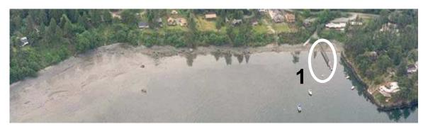
1. Dock (in use) with 14 creosote piles, each 180" x 12" dia. Plus ~ 450 feet of creosote timbers 4" x 12" in size plus 9 creosote timbers, each 72" x 12" x 12"
